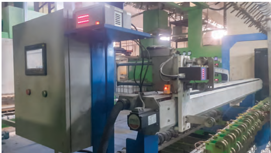
On Line Overall Dia recorder inbuilt in machine
